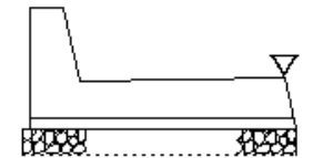
側溝工(L型街渠工)(LO型街渠工)
